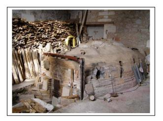
The Anagama or Dragon kiln, originally from the Far East, is intended for the production of utilitarian pottery and is built half buried into a slope in the ground. The kiln is filled throughout by flames which lick the pots placed on the steps within. The kiln can reach extreme temperatures  $(1350^{\circ}C-1400^{\circ}C)$ .
